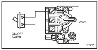
Fig. 10 Remote switch wiring.
